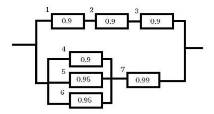
Define event  $E_i$ ="component *i* works". We decompose the circuit into sub-circuits. Consider the components 1, 2 and 3 which are assembled into series. We denote this component as 8. Thus,
