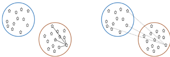
Figure 18. Distance to points in own clusters (left, smaller is better) and to points in other clusters (right, larger is better).
